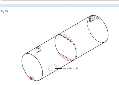
For tanks, vents should be diametrically opposite and at least 50mm in diameter. Internal baffles should be cropped top and bottom. Lifting lugs are required as indicated. It should be possible to view the baffles through either the vent holes or an inspection hole – the placement of the inspection hole should be discussed with the galvanizer.
