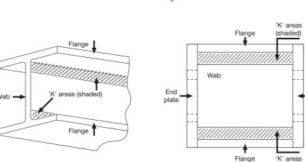
In circumstances where, due to design restrictions, general design guidance (as set out above) cannot be followed and the introduction of holes or other fabrication features into the 'K' areas of a section (where the web and flange meet) is unavoidable, please consult GA to discuss how best to finalise the design of the fabrication.
