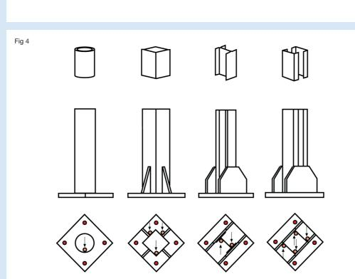
Alternative designs for venting sections fixed to base plates.
