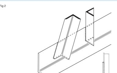
Angle bracings should, if possible, be stopped short of the main boom flange.
