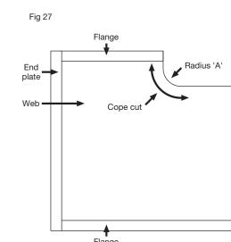
Cope cutting of beams is a common feature in modern steel construction. For optimum results during galvanizing, where flame-cut copes have
