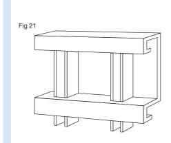
Use of symmetrical sections minimises distortion during hot dip galvanizing. Avoid combinations of thick and thin materials or where this cannot be avoided bolt together after individually hot dip galvanizing.
