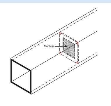
Internal diaphragms in large box sections should have cropped corners and a "manhole". Internal diaphragms on small box sections should
