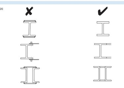
Welded joints should be continuous if they are not enclosing an otherwise unvented surface. Bolted joints are best made after galvanizing.
